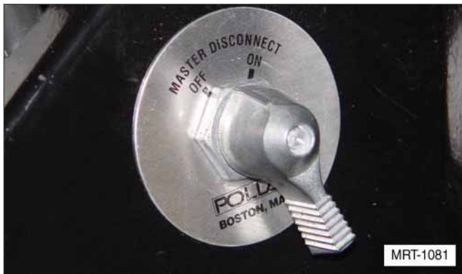
Cut-off switch mounted in cab of truck.
