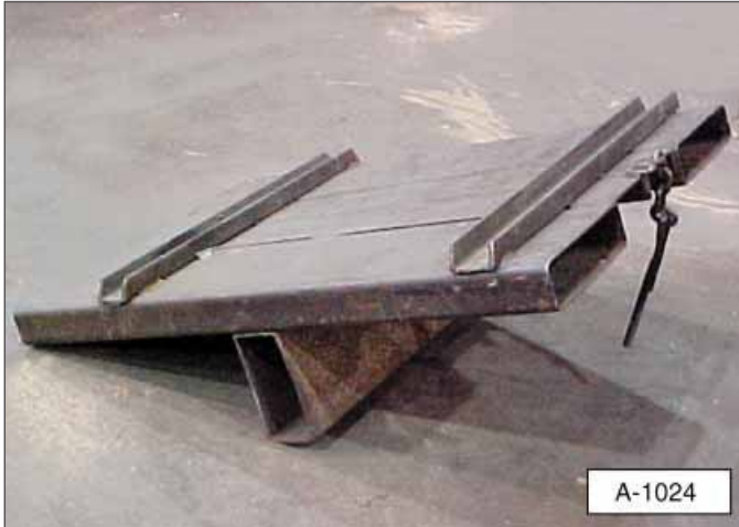
Installer-built Lifting Device.
