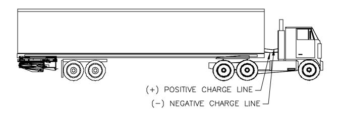
The Maintenance Minder 2<sup>®</sup> Controller requires a minimum of 10 volts to start and 8 volts to continue running the LPR lift gate. Power unit solenoid valves will require 10.5 volts to operate the coils. Utilization of a single positive cable often does not provide a sufficient ground for the charging circuit. Therefore, our recommendation for grounding tractor/trailers with the LPR gate is as follows:
