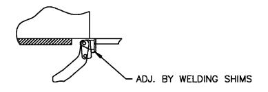
View with platform unfolded and in the full up position. *Caution:* Attach ground to stop blocks before welding.
