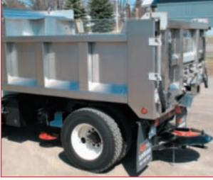
When spreading, the Flo'N Dump UNI-BODY has the lowest center of gravity of any multi-purpose body. A lower center of gravity makes the Uni-Body stable and safe on icy winter roads.
