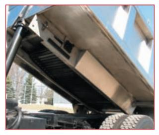
The conveyor combined with the trapezoidal longitudinals and a crossmemberless AR-400 floor, make for a very strong, efficient, and low maintenance multi-purpose dump body.
