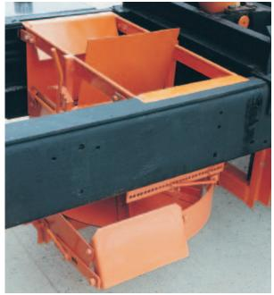
Optional Front Spread Model features exclusive chassis frame chute. This chute allows precise material applications – from spreading of all material under the truck to all material to the left lane of the truck or any combination in between.
