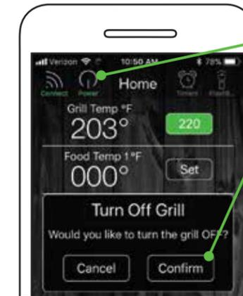
**OFF:** Tap the Power button, then press Confirm. The grill will cycle into Fan Mode.
