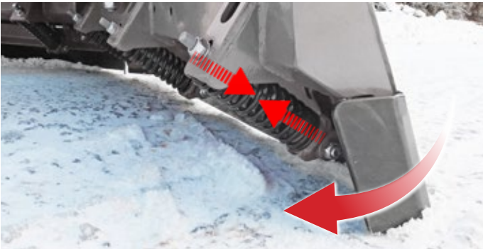
Cutting edge with trip springs
