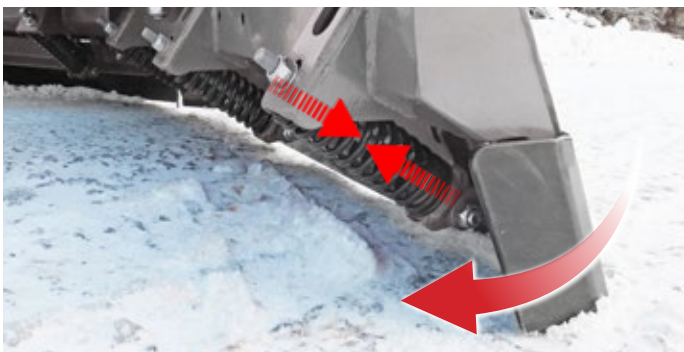
Cutting edge with trip springs
