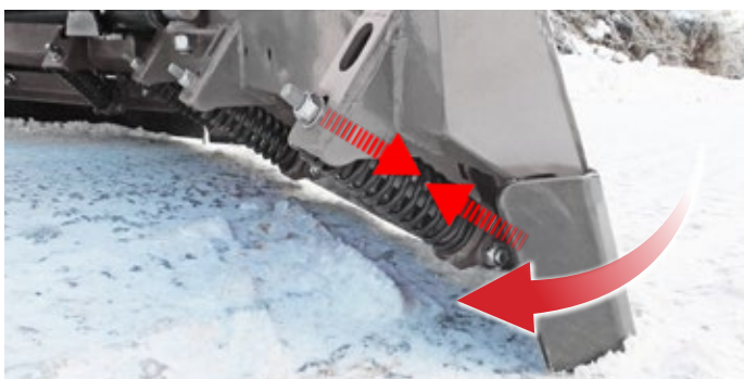
Cutting edge with trip springs
