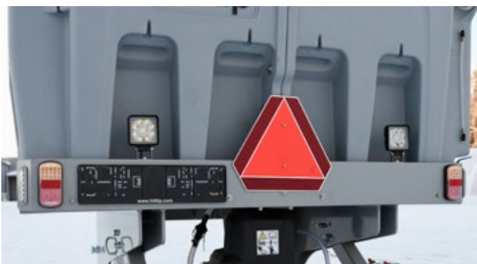
Optional LED work lights, strobe lights and LED stop/tail/brake light kit for 1200-1900 TR
