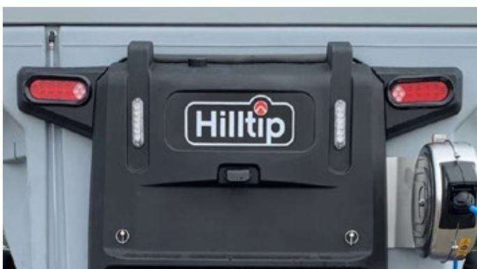
LED Stop/Tail/Brake lights and strobe lights
