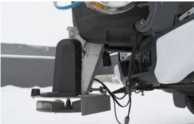
Stainless steel flip-up chute designed for spreading salt with high humidity
