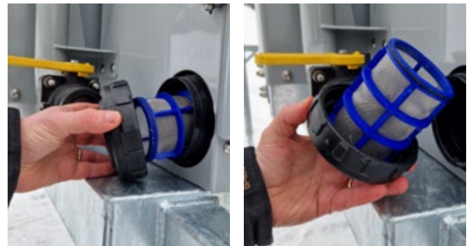
Unscrew the cap to check the filter
