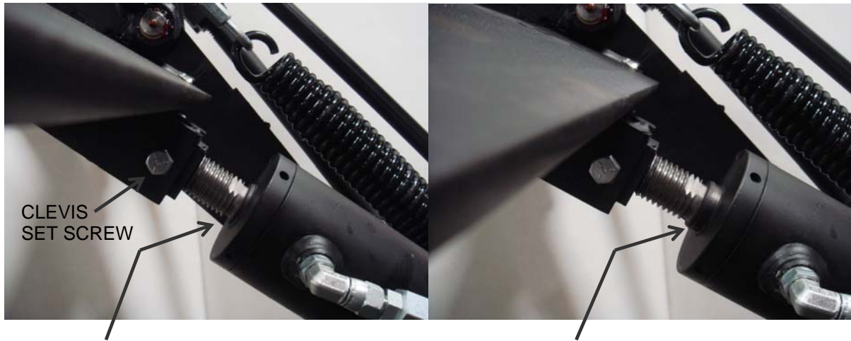
CYL ROD RETRACTED, DO NOT FORCE TRUNNION TUBE LOWER
