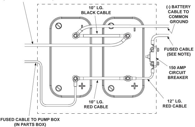
12 VOLT BATTERY CONNECTIONS FOR 12 VOLT POWER FIG. 30-1
