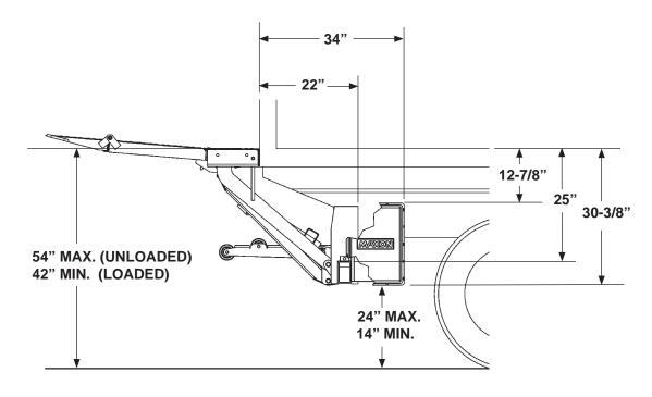
**CLEARANCES FOR TE-15 & TE-20 HIGH BED INSTALLATION (PAINTED)** FIG. 11-1
