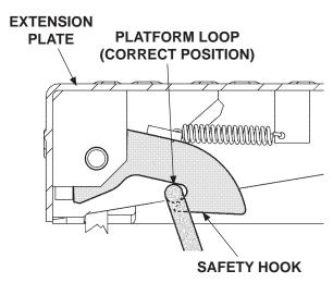
PLATFORM LOOP SHOWN HOOKED IN CORRECT POSITION FIG. 55-1
