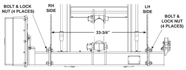
**BOLT-ON MOUNTING PLATES 33-3/4" (GALVANIZED)** (REAR VIEW OF LIFTGATE) FIG. 21-2
