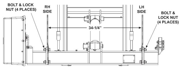
**BOLT-ON MOUNTING PLATES 34-1/4" (GALVANIZED)** (REAR VIEW OF LIFTGATE) FIG. 21-1
