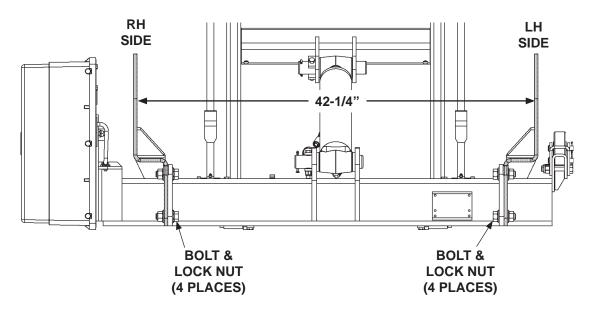
**BOLT-ON MOUNTING PLATES 42-1/4" (GALVANIZED)** (REAR VIEW OF LIFTGATE) FIG. 22-1
