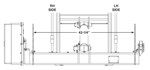
WELD-ON MOUNTING PLATES (PAINTED) TEMPORARILY BOLTED AS SHOWN (REAR VIEW OF LIFTGATE) FIG. 22-2
