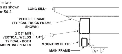
MOUNTING PLATE WELDED TO TRUCK FRAME & MAIN FRAME FIG. 54-1
