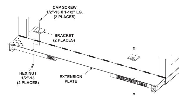
**BOLTING ON INSTALLATION BRACKETS** FIG. 20-1
