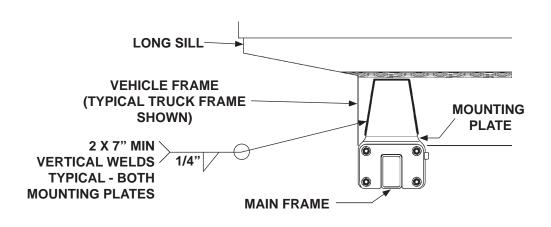
MOUNTING PLATE WELDED TO TRUCK FRAME & BOLTED TO MAIN FRAME FIG. 54-2
