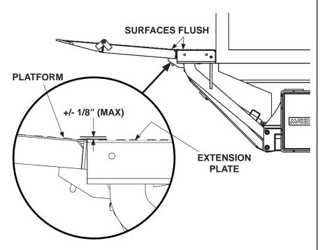
MAXIMUM DIFFERENCE IN HEIGHT FOR TOP OF PLATFORM & EXTENSION PLATE (RH VIEW) FIG. 48-1
