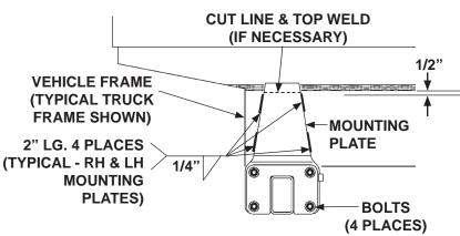
7. Clamp both mounting plates to vehicle frame. Weld the mounting plates to vehicle frame as shown in FIG. 25-2. Remove clamps.
