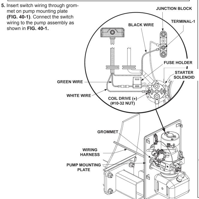
CONTROL SWITCH CONNECTED TO GD PUMP ASSEMBLY FIG. 40-1
