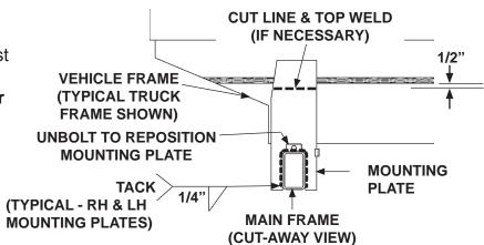
REPOSITIONING PAINTED MOUNTING PLATE (RH SIDE SHOWN) FIG. 24-1
