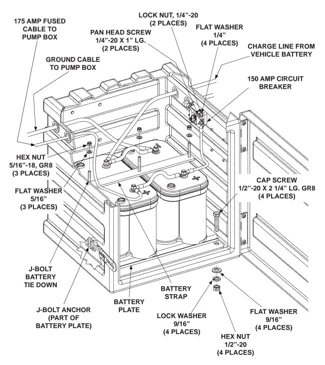
BATTERY BOX ASSEMBLY (12 VOLT POWER CONNECTIONS SHOWN) FIG. 33-1
