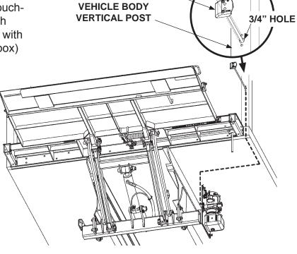
4. If necessary, use clamps and self-tapping screws (parts box) to secure switch cable to vehicle under-body and frame (FIG. 39-2).
