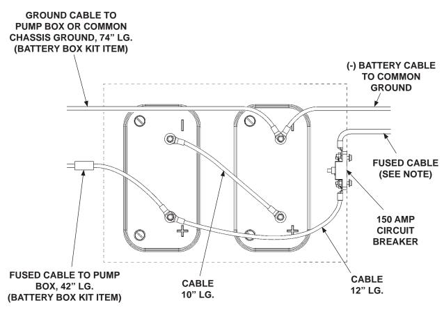
12 VOLT BATTERY CONNECTIONS **FOR 24 VOLT POWER** FIG. 31-1
