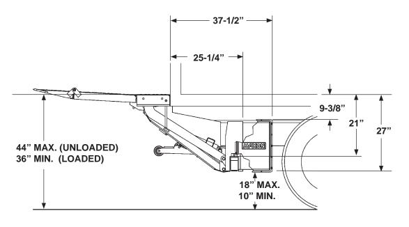
**CLEARANCES FOR TE-15 & TE-20 LOW BED INSTALLATION (PAINTED)** FIG. 11-2
