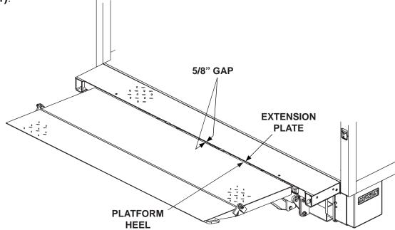
PLATFORM AT BED LEVEL WITH 5/8" GAP **BETWEEN HEEL & EXTENSION PLATE** FIG. 47-1
