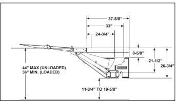
TE-25L/TE-30L Lift Dimensions and Mounting Requirements
