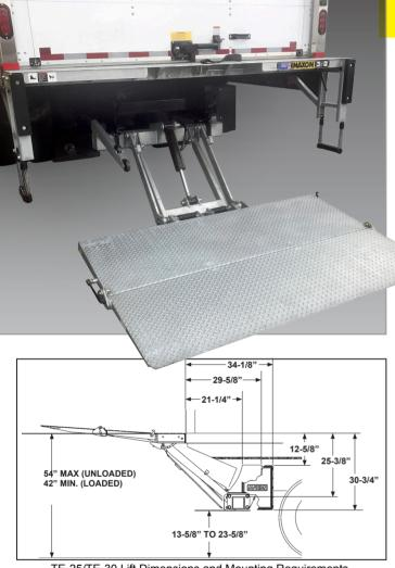
TE-25/TE-30 Lift Dimensions and Mounting Requirements
