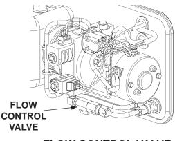
FLOW CONTROL VALVE (POWER DOWN) FIG. 47-2
