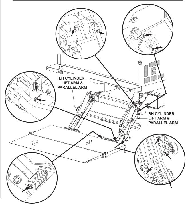
TE-33 LUBRICATION DIAGRAM FIG. 12-1
