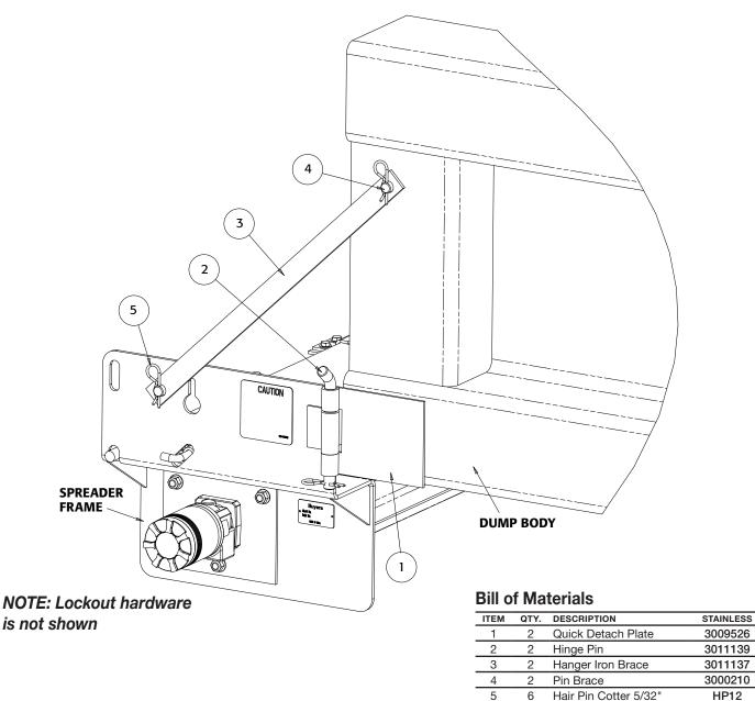
**E.** Weld the (2) pin braces (Item 4) to the dump body sides, all around.
