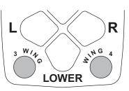
The two round buttons located to the left and right of the LOWER button move either wing independently of the other as described in the following table.
