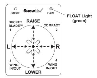
Moving the control lever straight up and down or from side to side on the control body will result in the blade movements described in the following tables.
