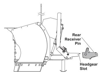
2. Hold down the lock lever and move the hitch pin handle out of the handle lock notch, allowing the spring to move the hitch pin handle forward.
