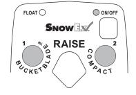
The two round buttons located to the left and right of the RAISE button move both wings at the same time into the blade positions described in the following table.
