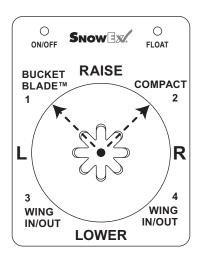
Moving the control lever from the center position toward the words "BUCKET BLADE" or "COMPACT" on the face of the control body will cause both wings to move at the same time into the following blade positions.
