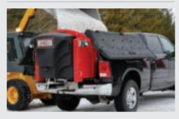
The overlapping poly hopper covers shield de-icing material from the elements, seal out moisture and act as spillguards to protect the truck from material overflow during loading.
